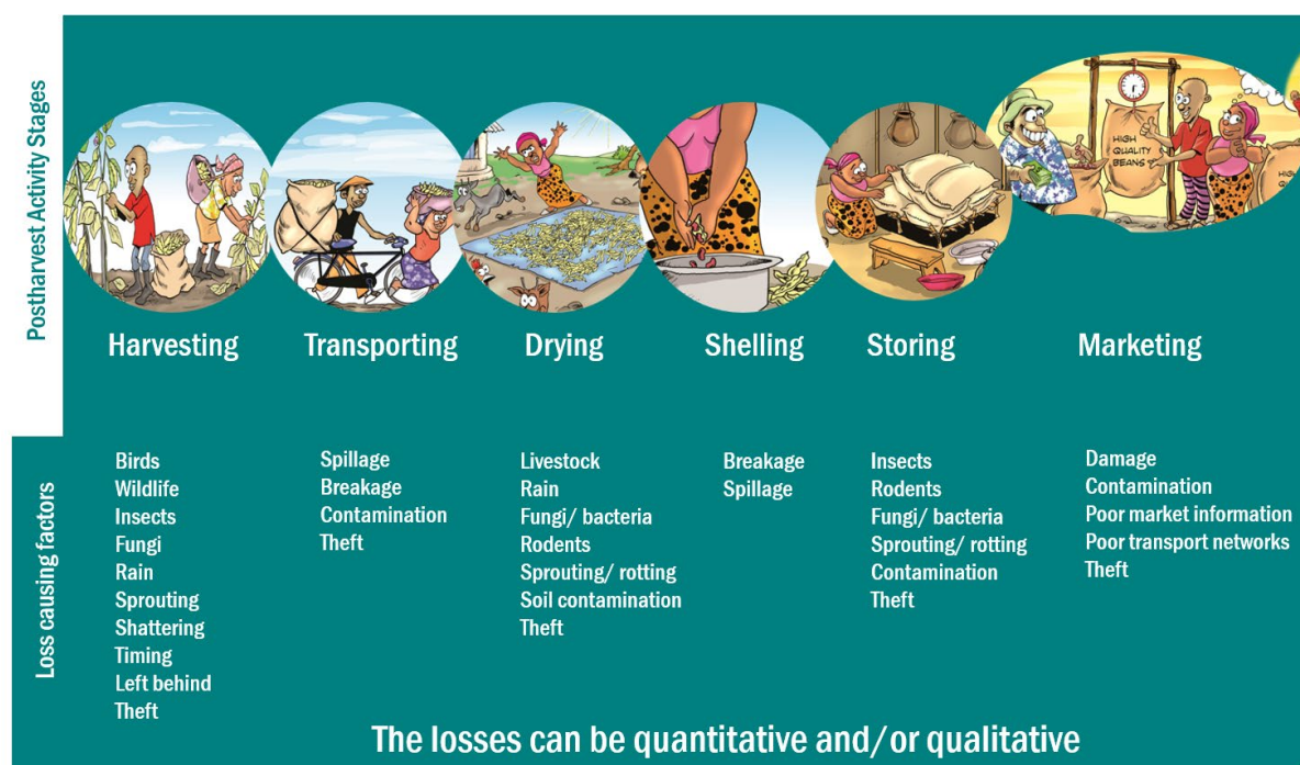
Figure 1. Grain postharvest activity stages and typical loss causing factors at each stage
